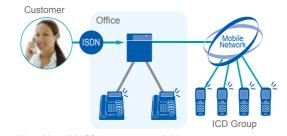
Note:Max 128 ICD groups are available. KX-TDA0920 SD Memory Card is required. Feature is not available with Analogue CO. This function is only available on ISDN lines
